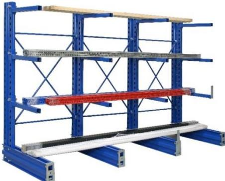
Cantilever racking is the most popular storage mechanism for long items including pipes, beams and rods made of metal, plastic or wood among other materials. The system basically consists set of uprights coupled with horizontal beams at the base that balances the rack. Cross bars between the uprights strengthens the stability of the entire storage system. A series of arms attached to the uprights bear the load of the items placed. The arms can be planned slightly inclined towards
