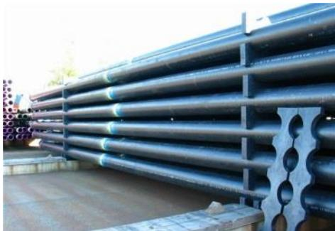
Pipe carriers offer an effective way of densely storing pipes on the ground. This system also supports the need wherein pipe-to-pipe contact should be avoided. A series of carriers are used to arrange pipes in an array. Pipes are typically handled using fork lift or cranes. Rolling of pipes and hammering of stop-chocks is avoided that provides additional safety to the entire setup.
